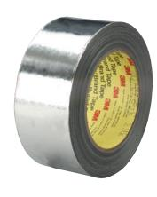
Strong and flexible, our 3M™ High Temperature Aluminium Foil/Glass Cloth Tape 363 consists of an aluminium foil, glass cloth backing combined with a pressure sensitive silicone adhesive. Ideal for use as a protective wrap for heat sensitive instruments exposed to movement and vibration.
