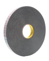
A thick, grey, double-coated acrylic foam tape with paper liner. The multi-purpose acrylic adhesive on both sides bonds to a broad range of high and medium surface energy substrates including metals, glass and a wide variety of paints and plastics. The conformable foam provides good contact between substrates even when they are slightly mismatched. Fast and easy-to-use permanent bonding method provides high strength and long-term durability
