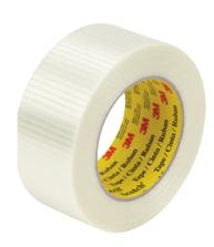
A speciality packaging tape reinforced with continuous glass yarns in both the longitudinal and transverse direction along with a biaxially oriented polypropylene backing. This backing provides good abrasion, moisture and scuff resistance. The adhesive is specifically formulated to provide good adhesion to a wide variety of surfaces including metallic, plastic, and fibreboard.
