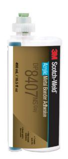
Grey structural adhesive with high overlap shear and peel strength with good impact resistance and durability. This adhesive was designed to bond permanently to bare metals with minimal surface preparation, but also bonds well to wide variety of other materials, including most plastics.
