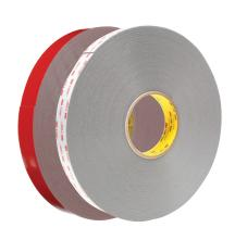
The multi-purpose acrylic adhesive on both sides bonds to a broad range of high and medium surface energy substrates including metals, glass and a wide variety of paints and plastics as well as plasticised vinyl. The conformable foam provides good contact between substrates even when they are slightly mismatched.
