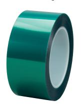
A general purpose polyester tape ideal for masking in high temperature applications. The translucent green backing is tear resistant. Coated with a silicone adhesive, this tape functions well in masking for powder coating to provide sharp paint lines. It removes cleanly and in one-piece from most surfaces, avoiding slivering and breaking.
