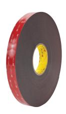
A modified acrylic adhesive on both sides bonds to a broad range of high, medium and medium/low surface energy substrates including metals, glass and a wide variety of plastics and paints, including many powder coated paints. The very conformable foam provides good contact between substrates even when they are slightly mismatched.
