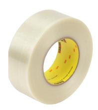
A high-performance transparent tape reinforced along its length with continuous fibreglass-yarn filaments, which gives the tape a very high tensile strength. The clear polyester backing provides excellent abrasion, moisture and scuff resistance.
