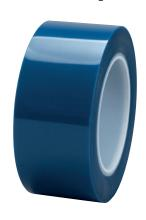
A general purpose polyester tape ideal for masking in high temperature applications. Coated with a silicone adhesive, this tape functions well in masking for powder coating and anodising to provide sharp paint lines. It removes cleanly and in one-piece from most surfaces, avoiding slivering and breaking.
