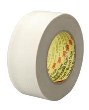
Constructed with a woven fibreglass backing, 3M<sup>™</sup> Glass Cloth Tape 361 features a pressure sensitive silicone adhesive for applications requiring high-temperature resistance, high adhesion and clean removal. It is often used for high temperature applications such as sealing ducts and as a back-up strip for submerged arc welding.
